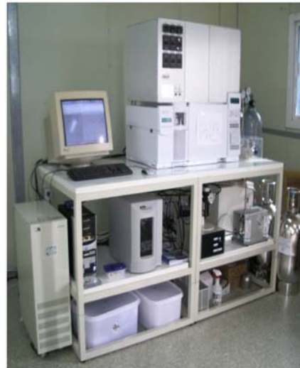
Medusa GC-MS: Measurement of ~40 species of halocarbons (CFCs, HCFCs, HFCs, PFCs, SF 6 , etc.) Operated since Nov., 2007
